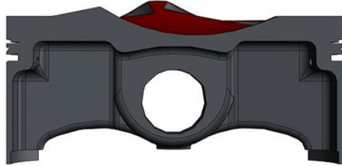
High Compression Deep Bowl Piston Design (Modified pentroof surface with 6mm deep bowl)
