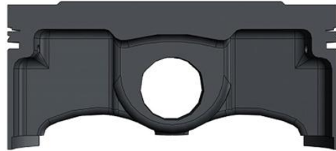
High Compression Flat Surface Piston Design (1mm head clearance with 1mm raised plateau)
